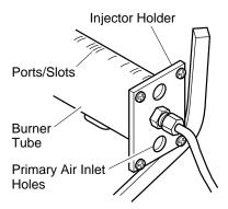
Figure 28 - Injector Holder On Outlet Burner Tube
